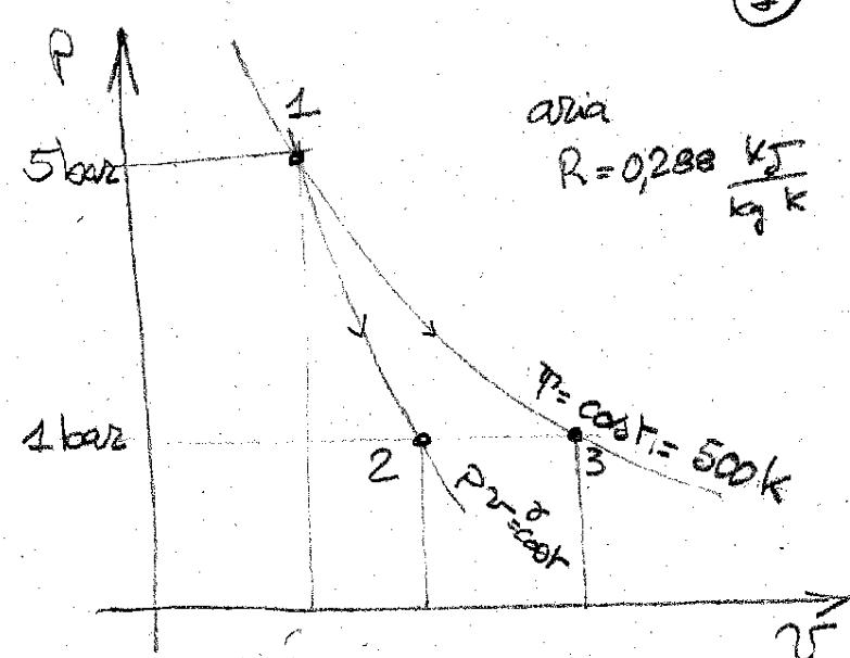
$$V_1 = \frac{RP_1}{R} = 0,288 \frac{\text{KJ}}{\text{kg K}} \cdot \frac{500 \text{ K}}{500 \text{ kPa}} \\ = 0,288 \frac{\text{m}^3}{\text{kg}}$$
