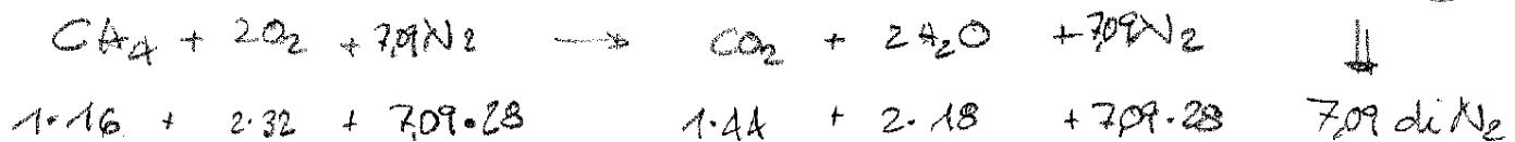
$$\dot{m}_{\text{aria}} + \dot{m}_{CH_4} = \dot{m}_{\text{fumi}}$$
