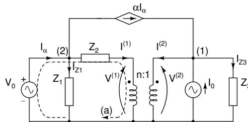
con  $Z_1 = 40j \Omega$ ,  $Z_2 = 20 + 40j \Omega$ ,  $Z_3 = 10 - 10j \Omega$ ,  $V_0 = 6 \cdot 10^{-1} \text{ V}$ ,  $I_0 = 3 \cdot 10^{-2} e^{j\pi/2} \text{ mA} = 3j \cdot 10^{-2} \text{ A}$ .
