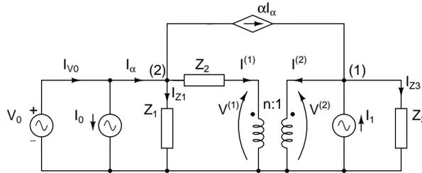
con  $Z_1 = 40j \text{ } \Omega$ ,  $Z_2 = 20 + 40j \text{ } \Omega$ ,  $Z_3 = 10 - 10j \text{ } \Omega$ ,  $V_0 = 6 \cdot 10^{-1} \text{ V}$ ,  $I_0 = 10^{-1} e^{-j\pi/2} = -j \cdot 10^{-1} \text{ A}$ ,  $I_1 = 3 \cdot 10^{-2} e^{j\pi/2} = 3j \cdot 10^{-2} \text{ A}$ .
