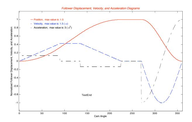
Draw the displacement schedule for a follower that rises through a total displacement of 20 mm with constant acceleration for 1/8th revolution, constant velocity for 1/4th revolution, and constant deceleration for 1/8th revolution of the cam. The cam then dwells for 1/4th revolution, and returns with simple harmonic motion in 1/4th revolution of the cam.
