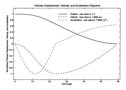
Assume that s is the cam-follower displacement and  $\theta$  is the cam rotation. The rise is 1.0 cm after 1.0 radian of rotation, and the rise begins and ends at a dwell. The displacement equation for the follower during the rise period is
