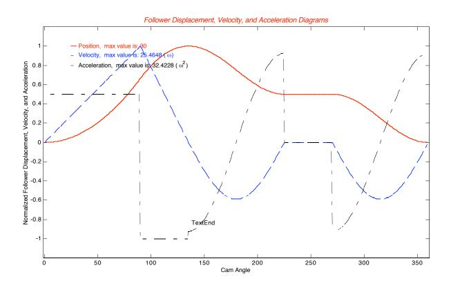
Draw the displacement schedule for a follower that rises through a total displacement of 3 inches with cycloidal motion in 120 degrees of cam rotation. The follower then dwells for  $90^{\circ}$  and returns to zero with simple harmonic motion in  $90^{\circ}$  of cam rotation. The follower then dwells for  $60^{\circ}$  before repeating the cycle.
