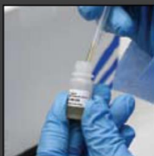
6. Draw the contents of the Sample Reagent Vial into a sterile transfer pipette.
