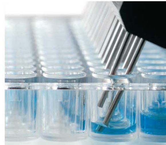
Proper position of manual washer needles for aspirating liquid
